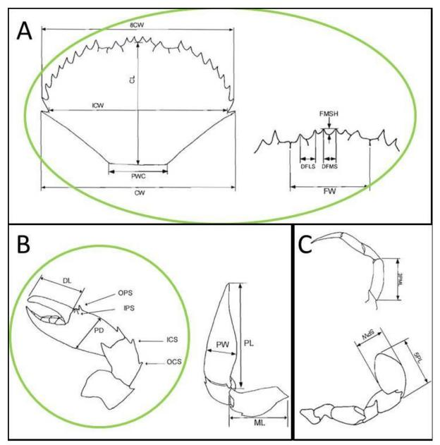
Figure 2. Standard sections for measurement on a crab. Green circles highlight the measurements that are most useful for species identification. A – carapace, B – cheliped, C — periopods.
