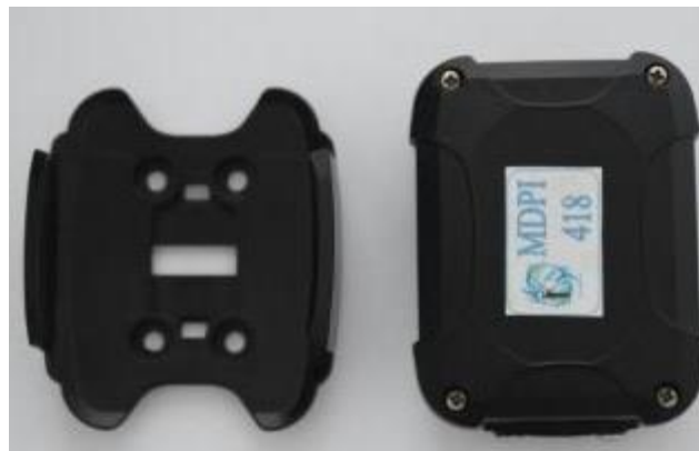
Figure 3. The back of the Spot Trace device. Left: the mounting bracket, right: the device asset number from MDPI.
