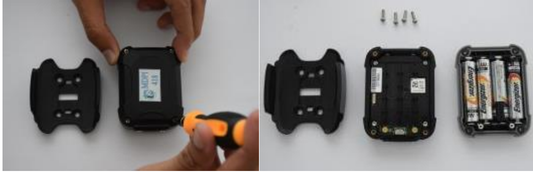
Figure 5. Opening the device (left). The device open with the batteries installed (right).
